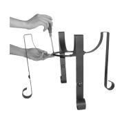
Align the holes of Small Ring (E) with the holes of each Leg (C), as shown. Loosely attach the ring to the legs using Bolt (F).
