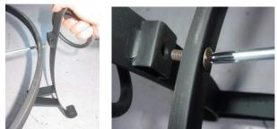
2. According to the same method above , assemble all stand legs but bolts cannot be twisted too tight .
