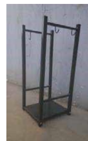
Assemble the steel base to the frames with bolts, washers, and nuts
