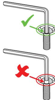
**Tip:** Always fully insert the hex key inside designated notch of the bolt.
