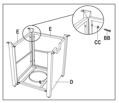
3. Attach Front Panel (D) and two Side Panels (E) to the legs using twelve M6 x 20mm Bolts (BB) and twelve Washers (CC).
