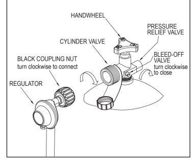
2. Ensure the propane cylinder is closed before connecting it to the fire pit by turning the handwheel clockwise. Attach the preassembled regulator from Table Top (B) to the cylinder valve by hand-tightening the coupling nut clockwise. Make sure the connection is tight and secure; do not use tools to tighten.
