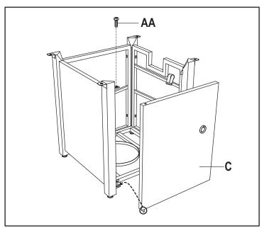
Insert the pin on the bottom of Door (C) into the axis hole on the bottom of Left Back Leg C. Attach Door (C) to Left Back Leg using one M6 x 12 Bolts (AA).
