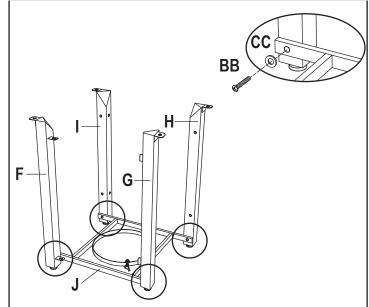
Attach Left Back Leg (F), Left Front Leg (G), Right Back Leg (I) and Right Front Leg (H) to Metal Stand (J) using four M6 x 20mm Bolts (BB) and four Washers (CC).
