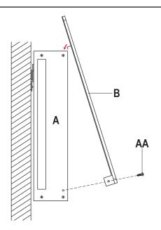
Lift Glass Front (B) into place, ensuring the 2 tabs on the top backside of the glass fit securely into the holes on the top of Firebox (A).
