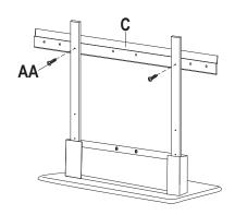
Secure Mounting Bracket (C) to the tabletop stand with two M4x8mm Screws (AA).
