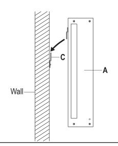
4 Hang Electric Firebox (A) on Mounting Bracket (C).
