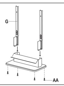
Attach the left and right Tabletop Supports (G) to the table top base (J) using 4 screws (AA).
