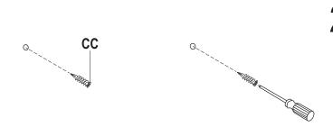
2 Insert the 2 self-drilling wall anchors (CC) into the wall where previously marked.
