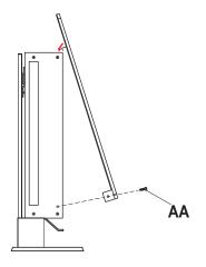
6 Lift Glass Front (B) into place, ensuring the 2 tabs on the top backside of the glass fit securely into the holes on the top of Firebox (A).
