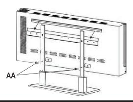
4 Hang Electric Firebox (A) on Mounting Bracket (C).
