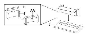
Attach Deflector (H) to Front (I) using two M4x8mm Screws (AA).
