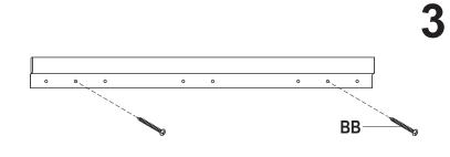
Secure Mounting Bracket (C) to the wall using two M4x35mm Screws (BB).
