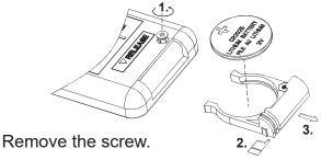
Press the release lever toward the center of the battery holder.
