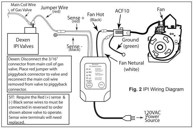
**WIRING NOTES**: When wiring an IPI system the Sense - (black) wire must be secure to a ground on the gas valve or to metal on the appliance for proper operation.
