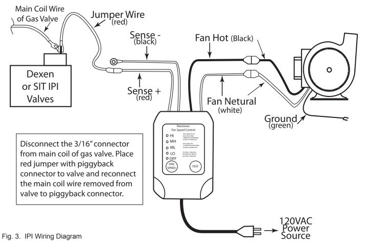
WIRING NOTES: <u>IPI System - When wiring an IPI system the Sense - (black) wire must be secure to a ground on the gas valve or to metal on the appliance for proper operation.</u>
