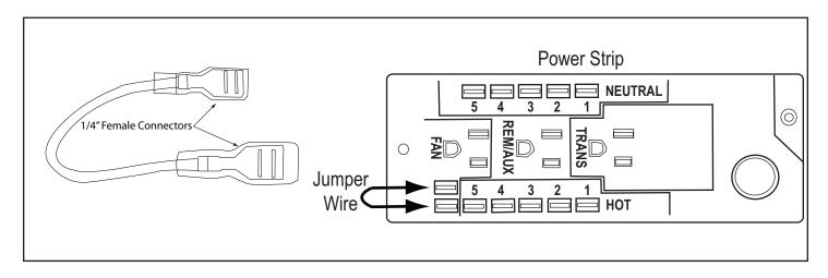
Fig. 4 Power strip jumper connection
