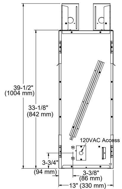
When utilizing the optional drain pan(ODLANAIG-48DP), please refer to installation manual for details.
