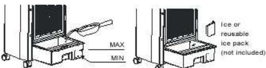
**NOTE:** Unit does NOT have a water-out indicator. Please add water when you hear a gurgling noise (the water pump trying to pump water).
