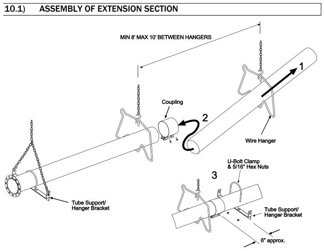
See typical assembly overview (Section 8.0)) for typical complete assembly. Assemble additional extension sections as required for all systems. (See Sections 7.0), and 8.0) for typical layout details.)
