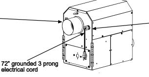
Liquid tight fitting must be tight to prevent ingress of moisture in harsh environments.
