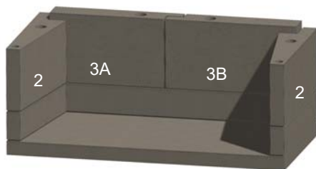
Figure 6. Lower Back Plates & Sidewalls
