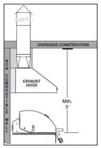
**Combustible Overhead Construction:** Exhaust hood required.
