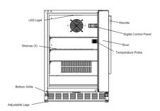
1. Position the unit to allow free air flow through the front grill.
