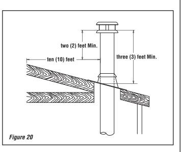
NOTE: 2" clearance to combustibles around chimney components required.
