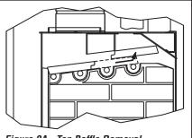
Figure 2A - Top Baffle Removal
