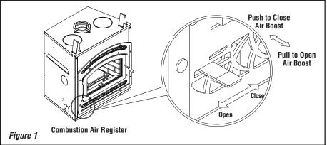
For instance, a long chimney will necessitate closing the damper more. To obtain the proper combustion, close the damper completely, then open it about 1/4" to 1/2". Three medium size pieces of wood should be burning on a bed of hot coals. The heat output will be approximately 30,000 BTU per hour and the loading time will be about every 3-4 hours. Softwoods may be burned using this method but the time will be substantially reduced.
