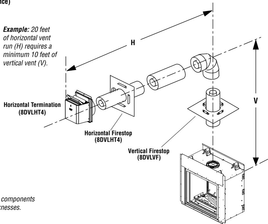
See Table 8 as an aid in selecting venting components for a particular range of exterior wall thicknesses.
