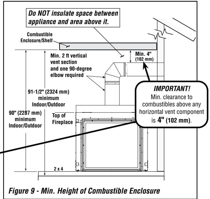
**Figure 9 - Min. Height of Combustible Enclosure**
