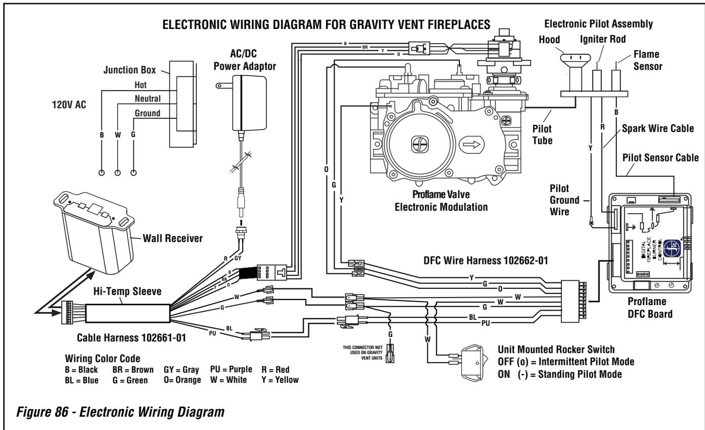
Figure 86 - Electronic Wiring Diagram
