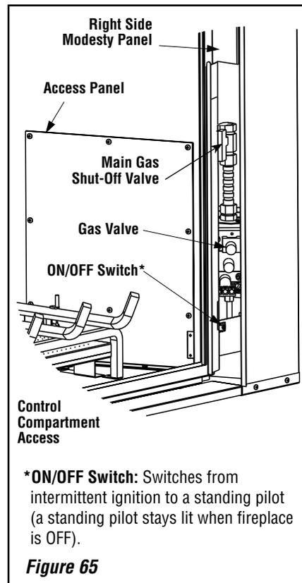
\*ON/OFF Switch: Switches from intermittent ignition to a standing pilot (a standing pilot stays lit when fireplace is OFF).
