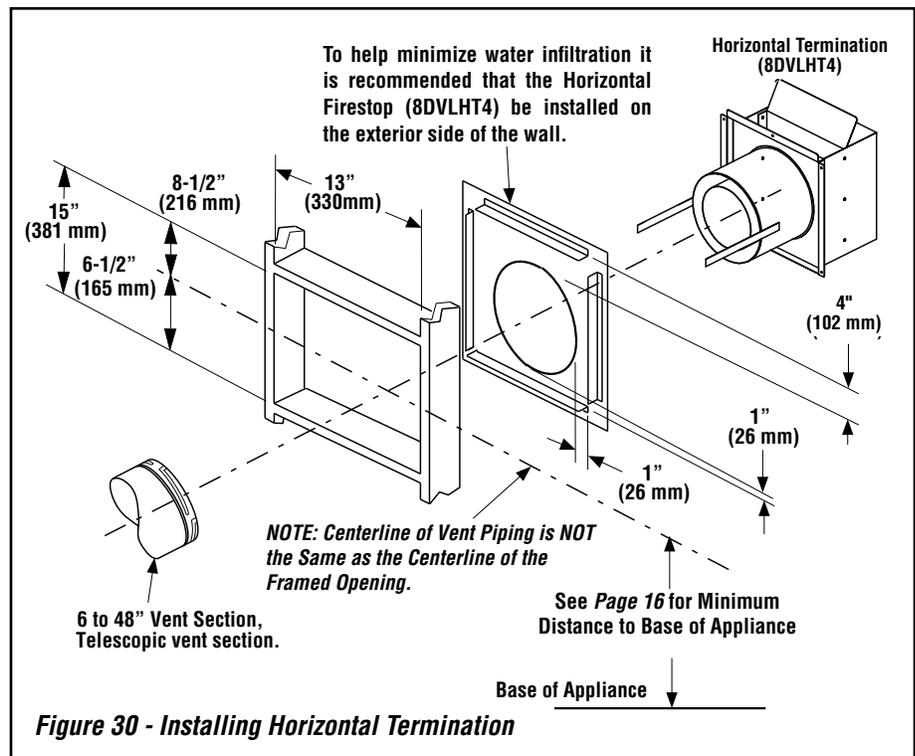
**Figure 30 - Installing Horizontal Termination**
