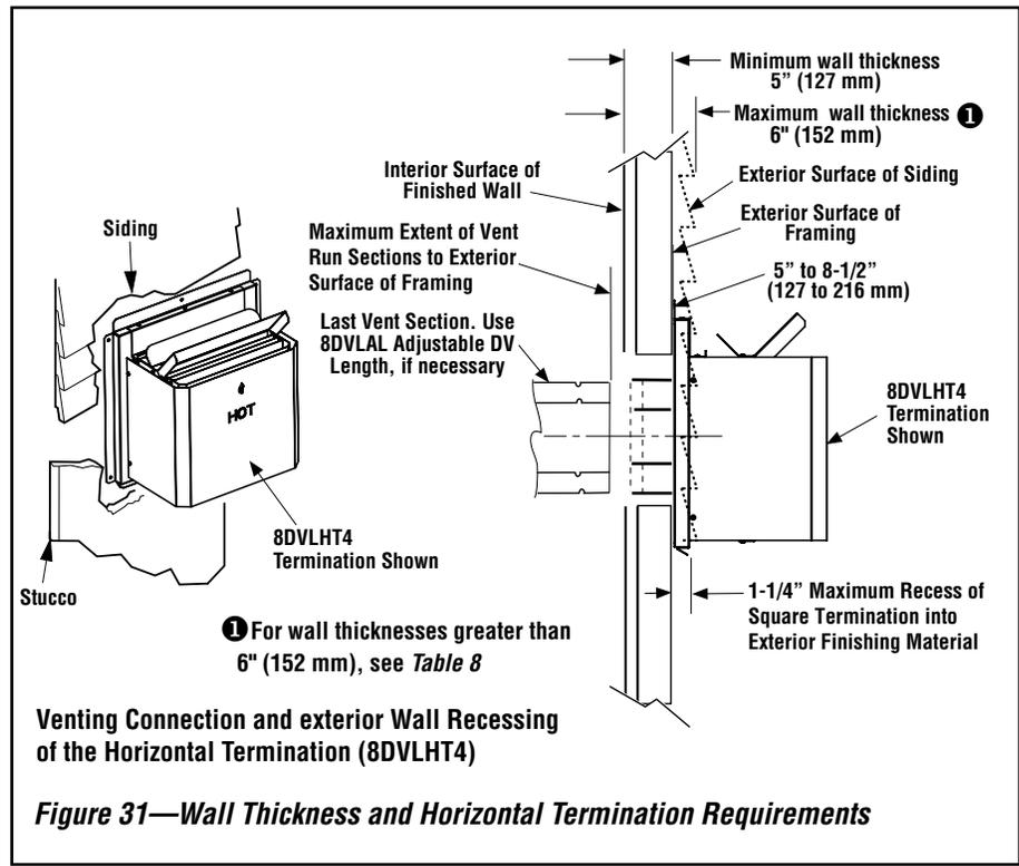
**Venting Connection and exterior Wall Recessing of the Horizontal Termination (8DVLHT4)**
