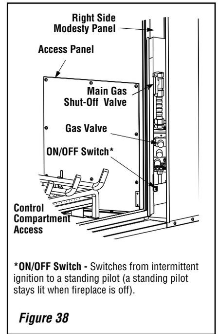
\*ON/OFF Switch - Switches from intermittent ignition to a standing pilot (a standing pilot stays lit when fireplace is off).
