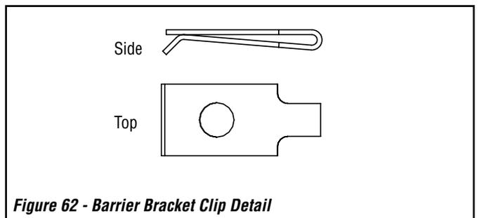
**Figure 62 - Barrier Bracket Clip Detail**
