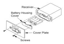
Figure 22 - Battery Install Remote Control Receiver
