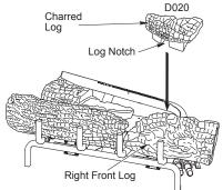
Figure 27 - Installing Charred Log
