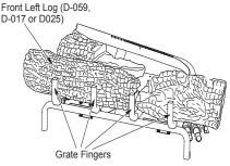
Figure 26 - Installing Front Left Log
