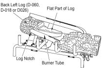
Figure 25 - Installing Back Left Log
