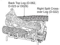
Figure 31 - Installing Back Top Log and Final Assembly
