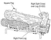
Figure 29 - Installing Right Split Crossover Log
