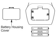
Figure 20 - Battery Install Hand-Held Remote Control
