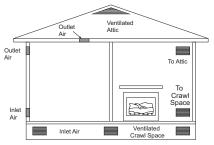
Figure 3 - Ventilation Air from Outdoors
