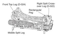
Figure 30 - Installing Large Middle Log
