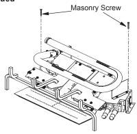
Figure 12 - Attaching Base to Fireplace Floor
