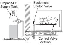
Figure 16 - Checking Gas Joints (Propane/LP Only)
