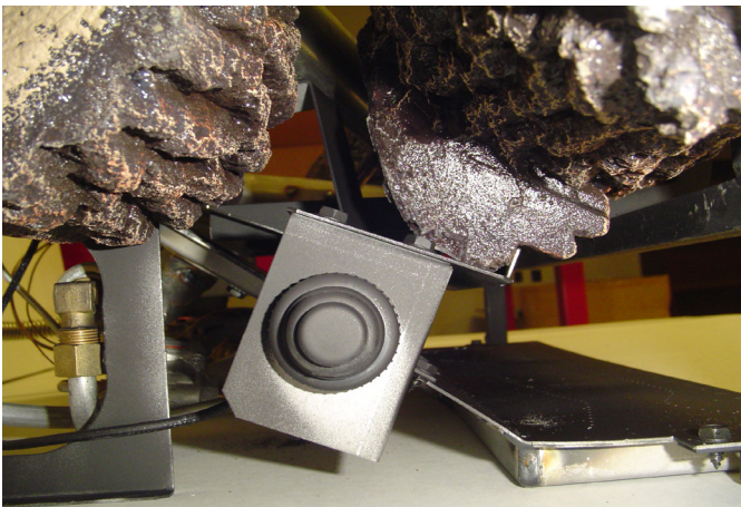
Figure 18A - Installing Front Left Log Side View
