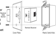
**NOTE**: The remote receiver will only respond to the transmitter when the 3-position slide button on the remote receiver is in the REMOTE position. If the system does not respond to the battery transmitter on initial use, see CODE SETTING SECTION, and recheck battery positions in the remote receiver.
