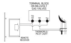
Operation of the remote receiver is similar to that of a thermostat in that both turn the gas on and off based on input signals. A thermostat's input signals are different temperatures. remote receiver's input signals come from the transmitter.
