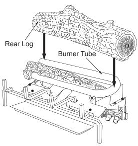
Figure 35 - Installing Rear Log
