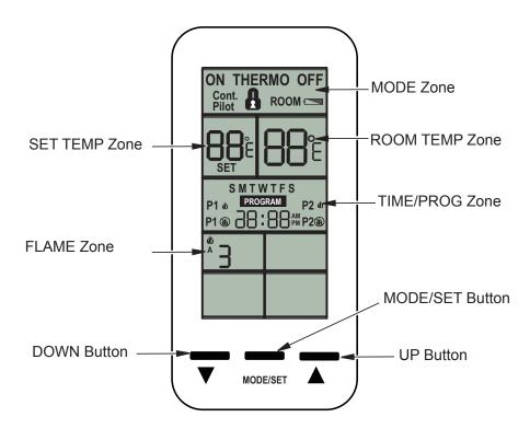
Figure 52 - Touch-Screen LCD and Button Layout
