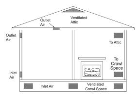
Figure 3 - Ventilation Air from Outdoors
