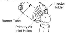
Figure 56 - Injector Holder On Outlet Burner Tube
