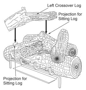
Figure 39 - Installing Left Crossover Log
