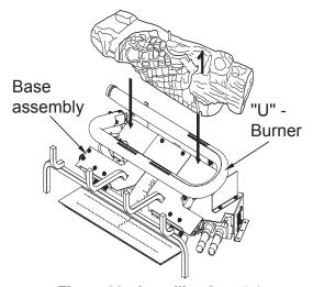
Figure 22 - Installing Log # 1
