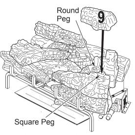
Figure 30 - Installing Log # 9
