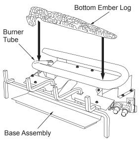
Figure 34 - Installing Bottom Ember Log
