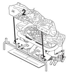
Figure 23 - Installing Log # 2
