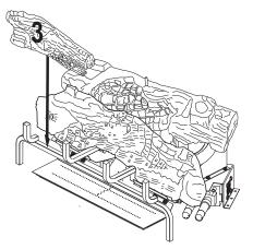
Figure 24 - Installing Log # 3
