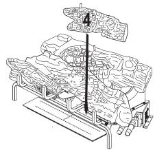
Figure 25 - Installing Log # 4
