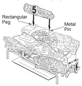
Figure 26 - Installing Log # 5
