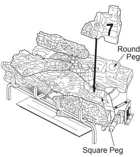
Figure 28 - Installing Log # 7
