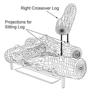
Figure 38 - Installing Right Crossover Log
