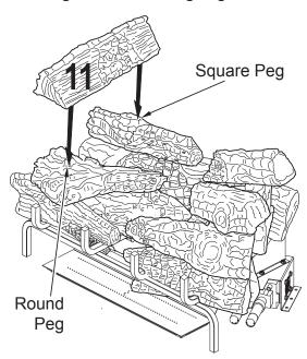
Figure 32 - Installing Log # 11
