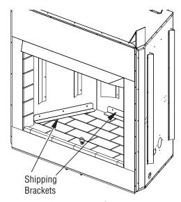
Figure 13 - Removing Shipping Brackets
