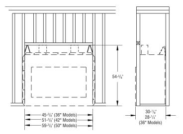
Figure 8 - Framing Dimensions
