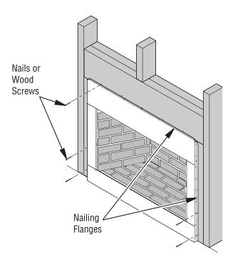
Figure 10 - Attaching Firebox to Wall Studs
