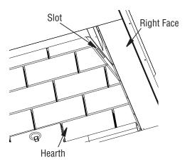
Figure 14 - Slots for Firebrick Walls
