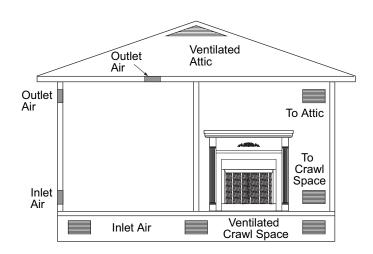
Figure 5 - Ventilation Air from Outdoors
