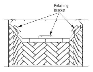
Figure 15 - Installing Side Walls
