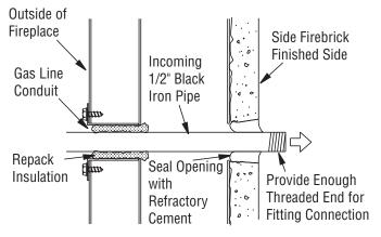
Figure 19 - Gas Line Installation
