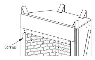
Figure 16 - Screw and Hood Placement
