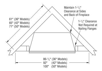
Figure 9 - Corner Installation
