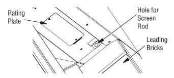
Figure 17 - Installing Fireplace Screen
