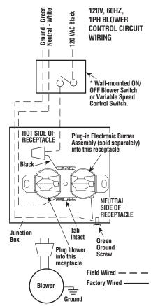
\*A ON/OFF Wall Switch is used with the FBK-100 kit (field provided; A Variable Speed Control (provided) is used with the FBK-200 kit. The installation of these kits also require a Junction Box / Electrical Kit (provided).
