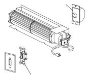
An locally sourced ON/OFF wall switch can be used with the FBK-100 models
