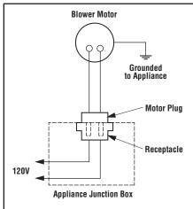
NOTE: If any of the original wire as supplied must be replaced, it must be replaced with type AWM 105 degree C - 14 gage wire.
