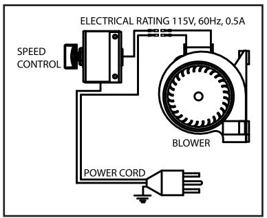
Figure 9: Blower Wiring Diagram.
