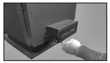
Figure 11: Installing the blower.
