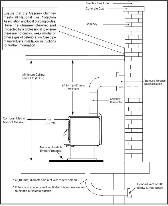
Figure 7: Venting to a masonry chimney.
