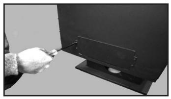
Figure 10: Remove the cover plate.
