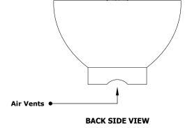
Fire Pit Material: GFRC Concrete Pan Material: 304 Stainless Steel Burner Material: 304 Stainless Steel
