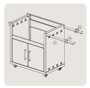
10. Assemble the side shelf to the brackets, as shown below.
