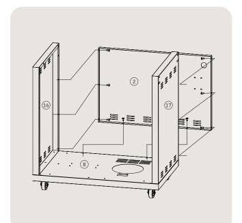
2. Use M5\*10 bolt (6pcs) to install the left side panel and ride side panel to the bottom panel.
