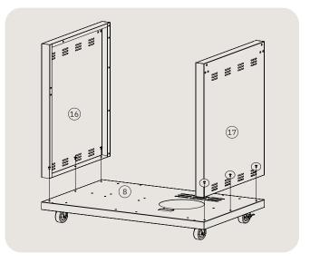
4. Use M5\*10 bolt (4pcs) to assemble the rear upper panel with the left side panel and right side panel.
