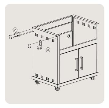
9. Use M6\*12 countersunk screws (6pcs) to install the side shelf left (14) and right (15) brackets to the ride side panel.
