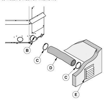
Figure 26: Fresh air intake kit installation
