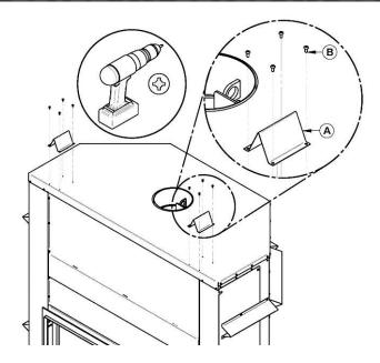
Figure 12: Installation of spacers
