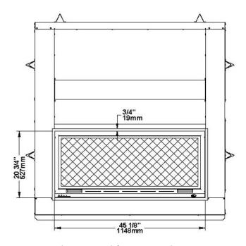
Figure 4: Straight masonry trim
