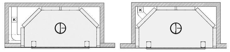
Figure 21: Fresh air intake - Side Installation
