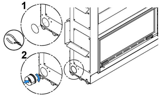
Figure 28: Adapter installation
