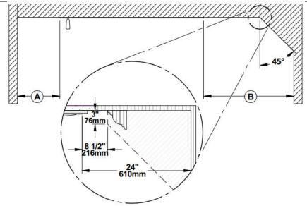
Figure 13: Clearances to combustible materials
