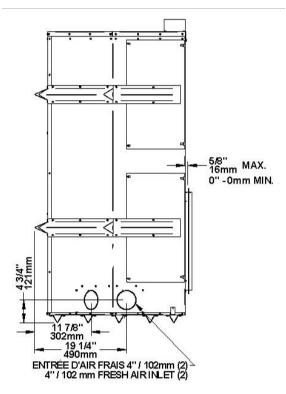
Figure 10 : Left Side Straight masonry trim
