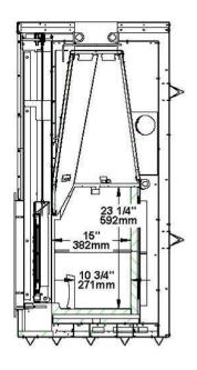
Figure 6 : Combustion chamber
