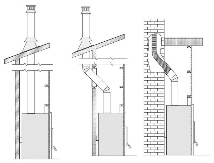
Figure 45: Straight Installation
