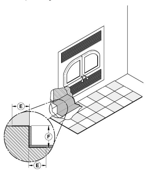
Figure 16: Raised base installation of 4"
