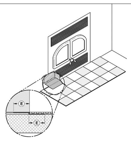
Figure 17: Installation Directly on the floor
