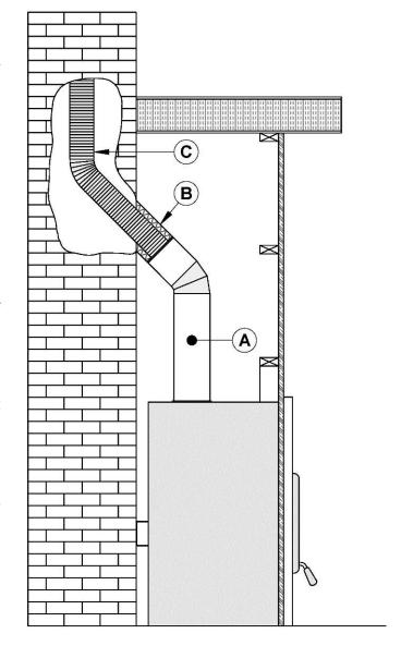
Figure 51: Masonry Chimney Installation
