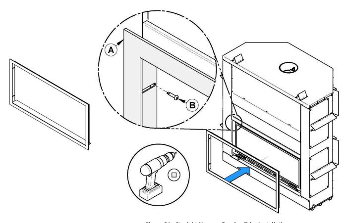
Figure 31 : Straight Narrow Overlap Trim Installation
