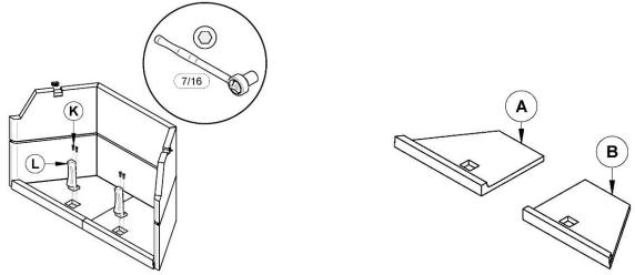
Figure 33: Andirons and Anchors bolts
