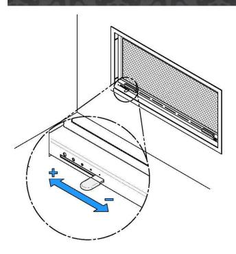
Figure 54: Air Intake Control
