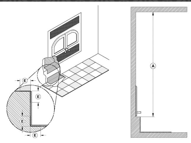
Figure 14 : Raised base installation of more than 4"
