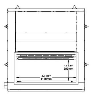
Figure 7 : Door Opening Straight narrow overlap faceplate
