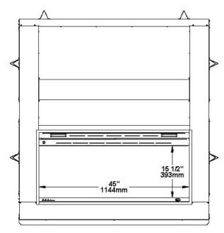
Figure 8 : Door Opening Straight masonry trim
