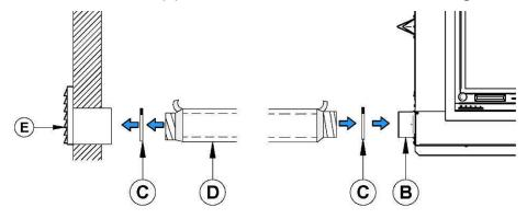
Figure 29: Fresh air intake installation
