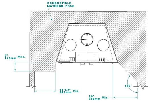
Figure #15: Chimney Enclosure
