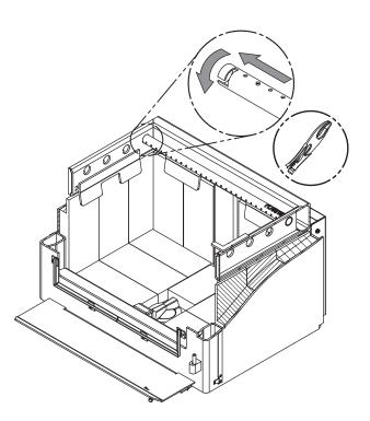
Note that secondary air tubes (B) can be replaced without removing the baffle board (A) and that all tubes are identical.
