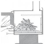
Then add two or three small pieces of firewood. Open the air intake control completely and ignite the newspaper. Leave the door slightly ajar. Once the fire has ignited, the door can be closed with the air control still fully open. When the kindling is almost completely burned, standard firewood pieces can be added.
