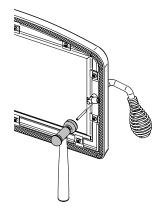
Reinstalling the retaining pin
