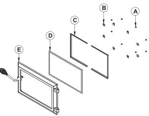
The two main causes of broken door glass are uneven placement in the door and overtightening the retaining screws.
