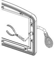
Removing the retaining pin
