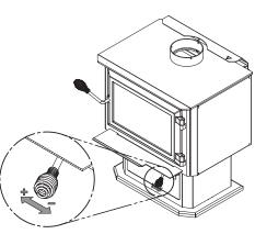
On the other hand, too much air can make the fire uncontrollable, creating very high temperatures in the unit as well as in the chimney and seriously damaging them. A reddish glow on the unit and on the chimney components indicates overheating. Excessive temperatures can cause a chimney fire.
