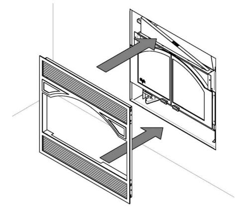
2. Firmly push the faceplate to the fireplace/wall finish. Using a power driver, secure the top and the bottom with 4 self-tapping screws (two on each side) provided with the fireplace owner's manual.
