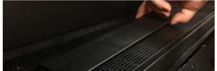
Figure 13.b Loosening the venturi
