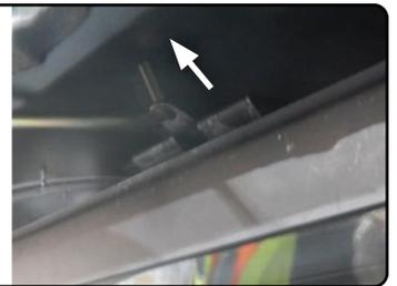
Figure 21.d Pull door latches
